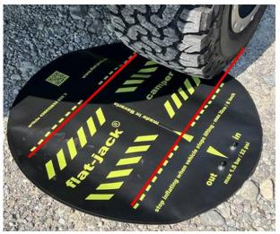
Image 6: Correct positioning of the flat-jack®
