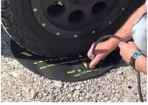
Image 11: Connecting the air pump
