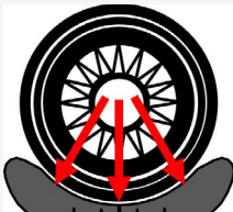
Large contact area with an even and low pressure to the rim
